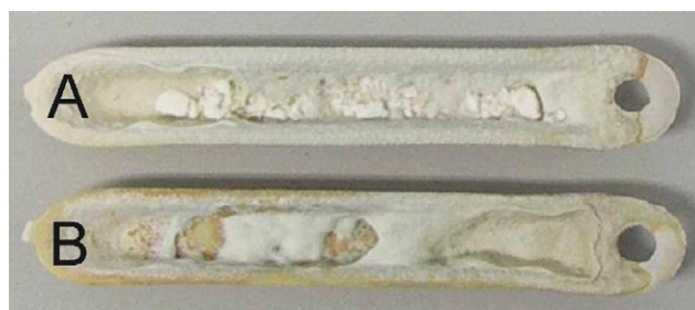
Fig. 7. Solidified LiOH melts after sample decomposition. (A) Without addition of 0.1 g of boric acid; (B) with addition of 0.1 g of boric acid.
